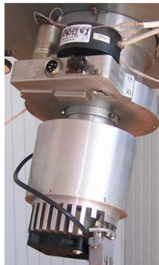
Image 1. Rotation system with CCD camera
